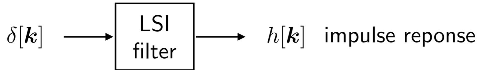
A discrete LSI filter is uniquely characterized by its impulse response, which is the **space-reversed** version of its mask:  $h[\mathbf{k}] = w[-\mathbf{k}]$
